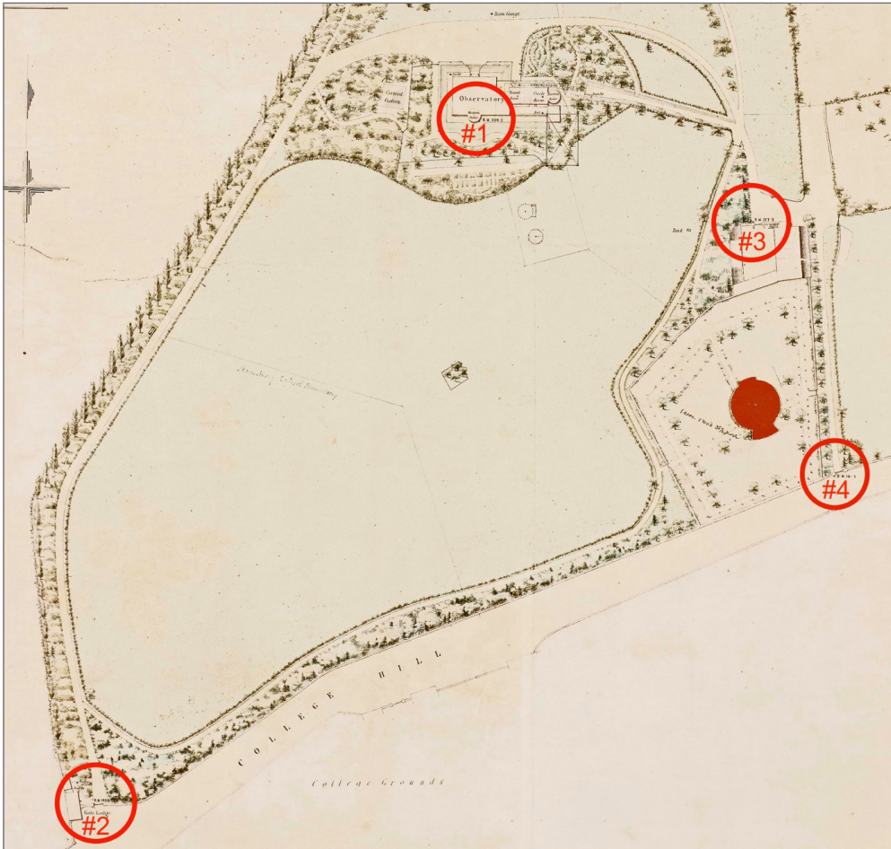
Figure 1. The four OSBMs shown on an OS map of the Observatory demesne commissioned by the Governors and Guardians of the Observatory in 1859 and held in Armagh Observatory. North is to the top. Nowadays only three survive, namely those near (1) the base of the Troughton telescope dome on the main building; (2) the foot of the western gate post of the main entrance to the Observatory grounds from College Hill; and (3) the base of the surviving western gate pillar of the entrance to the original coach house and stables, near the footpath leading downhill from the Observatory to what is now the Planetarium. The fourth benchmark, on a gate post adjacent to the Observatory demesne close to the c.1900 Urban District boundary near what later became the main entrance to the Planetarium, was lost during construction of the Planetarium during the mid-1960s. The filled symbol identifies the position of the first Planetarium building. Further information is given in Figure 2.
