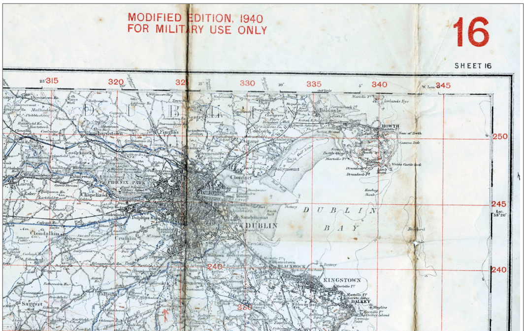
Fig. 4. Part of the first (1940) 'modified edition for military use only' of OSI 1:126,720 Sheet 16. A 5000-yard grid has been added to the black outline OSI half-inch map. (Author's copy).
